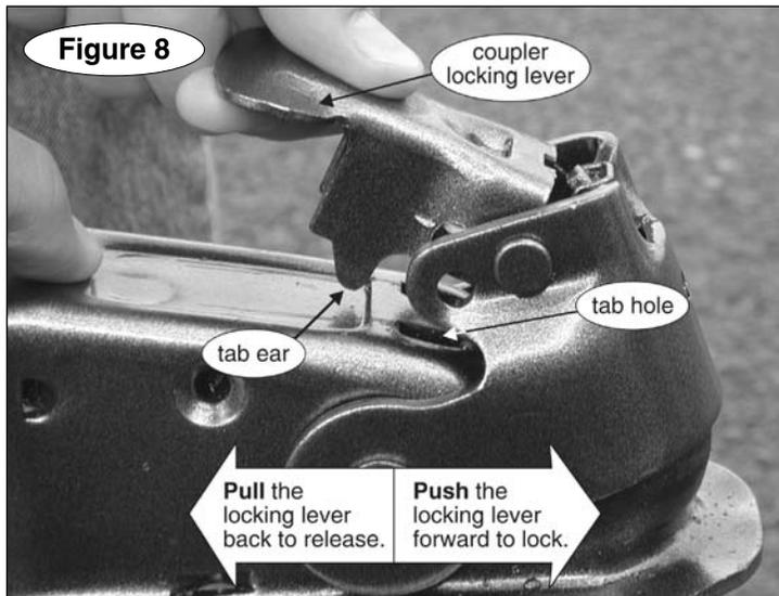
Now, lower the coupler over the hitch ball so that it completely covers it, and slide the coupler locking lever forward until it locks on the ball.
