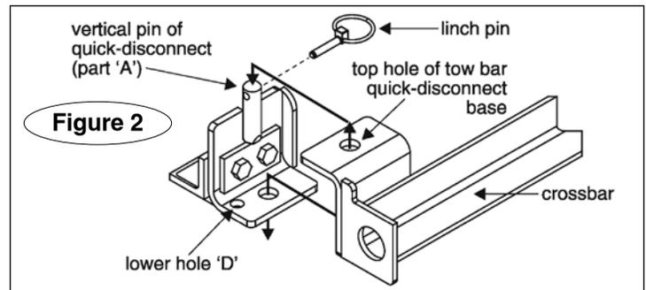
If they are attached too far to the left or the right, the tow bar will not be centered on the towed vehicle, which will cause excessive tire wear and other consequential, non-warranty damage.
